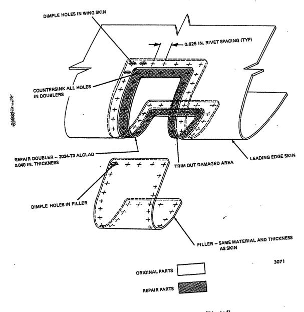
Leading Edge Repair (Riveted) Figure 801
