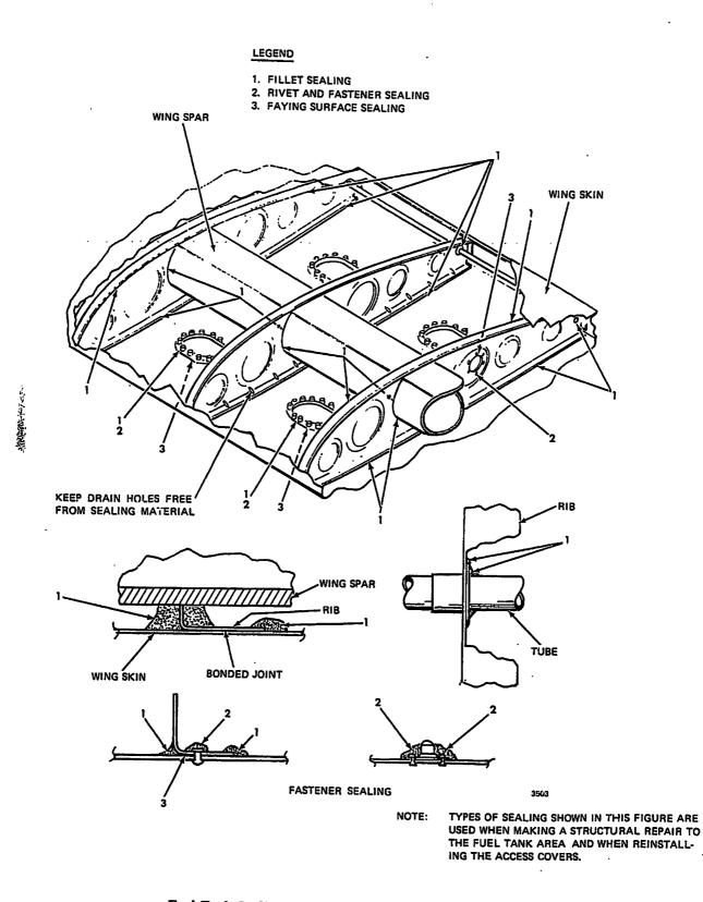
Fuel Tank Sealing - Model AA-5A (Optional) & AA-5B Figure 801 (Sheet 2 of 2)
