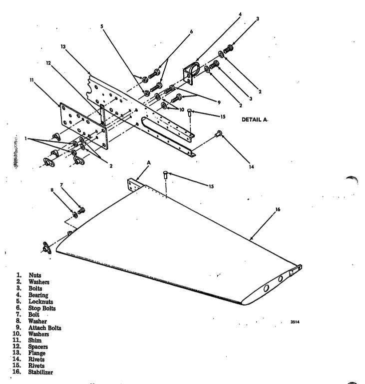
Horizontal Stabilizer Removal/Installation (AA-5 Aircraft) Figure 201
