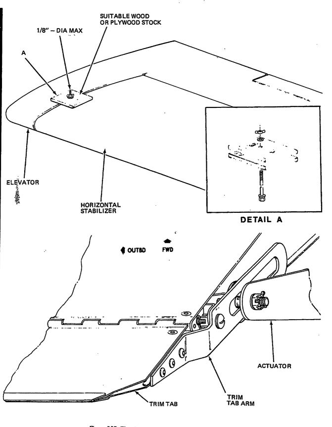
Figure 507. Elevator Trim Tab Free Play Measurement (Sheet 1 Of 2)
