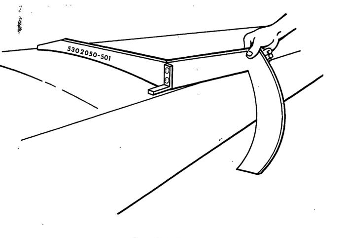
Elevator Rigging Fixture Figure 504
