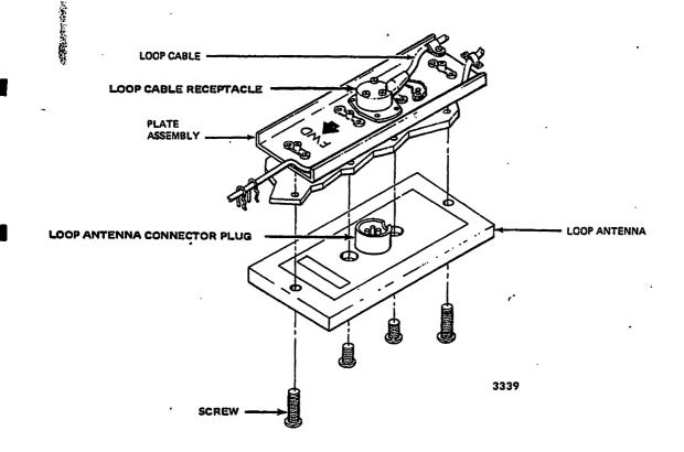
ADF Loop Antenna Installation Figure 201
