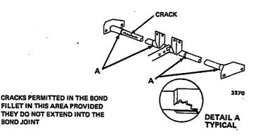
Torque Tube and Yoke Assembly Figure 205
