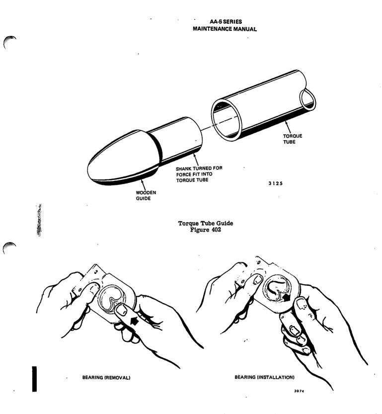
Aileron Bearing Removal/Installation Figure 403
