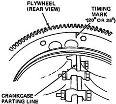
Advance Timing Alignment Figure 203 (3) Remove the plug from the bottom of the magneto.
