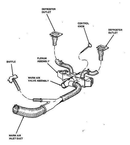
Defrosting System AA5-0001 through 0834 and AA5B-0001 through 0522 (Sheet 1 of 4) Figure 1
