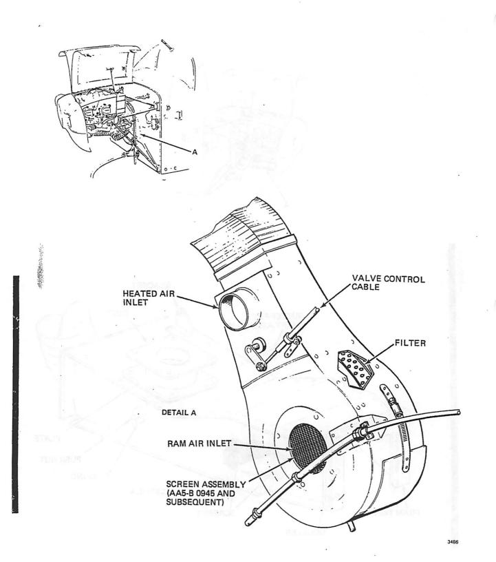
Carburetor Air Box Installation — AA-5B Figure 4
