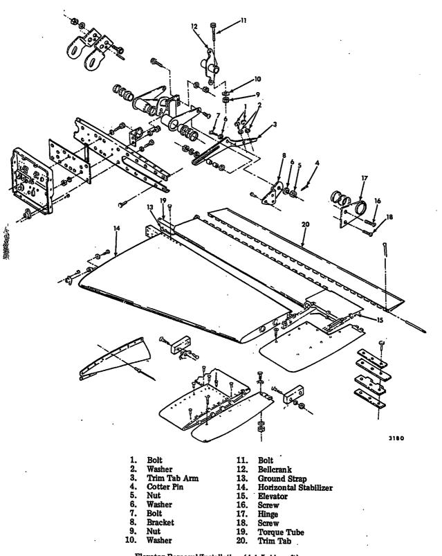
Elevator Removal/Installation (AA-5 Aircraft) Figure 401
