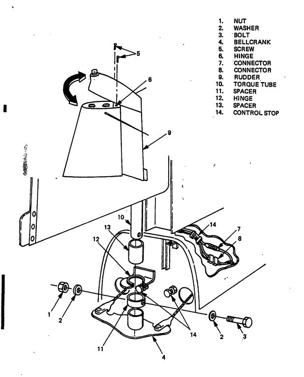
Rudder Removal/Installation Figure 401
