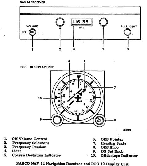
All operating controls for the NAV 14 and DGO 10 are mounted on their front panels and are identified in Figure 3.
