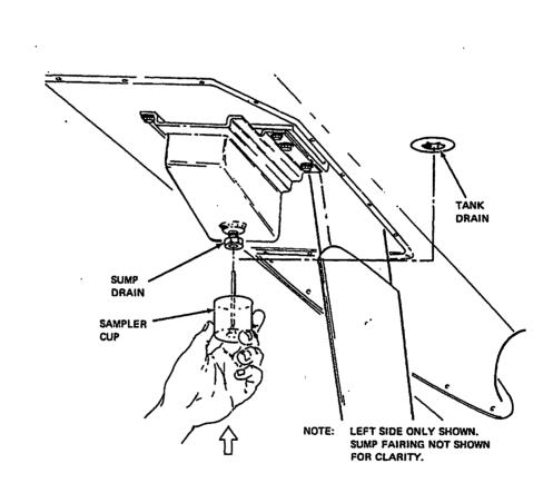
Fuel Sump and Fuel Tank Drain Operation Figure 201
