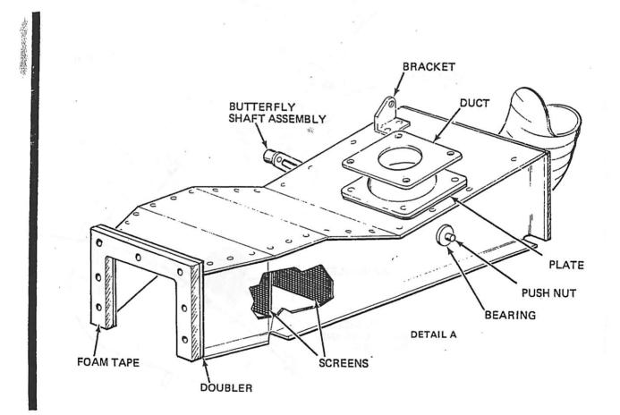
Carburetor Air Box Installation – AA5-0641 and Sub. and AA5A-0001 and Sub. Figure 3
