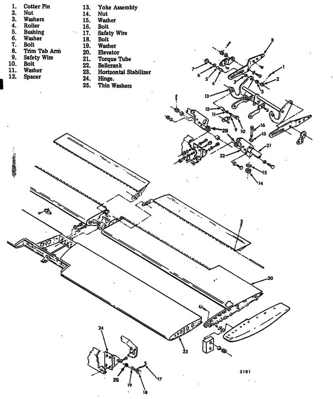
Elevator Removal/Installation (AA-5A and AA-5B Aircraft) Figure 402
