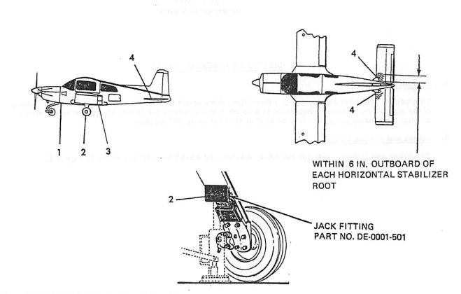
1. Front Lifting Point - Fuselage Station 51.
