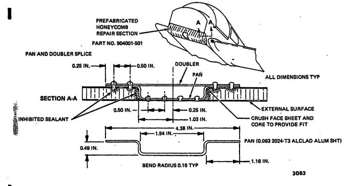
Honeycomb Repair — Forward Fuselage Section — (Flush Riveted) Figure 806
