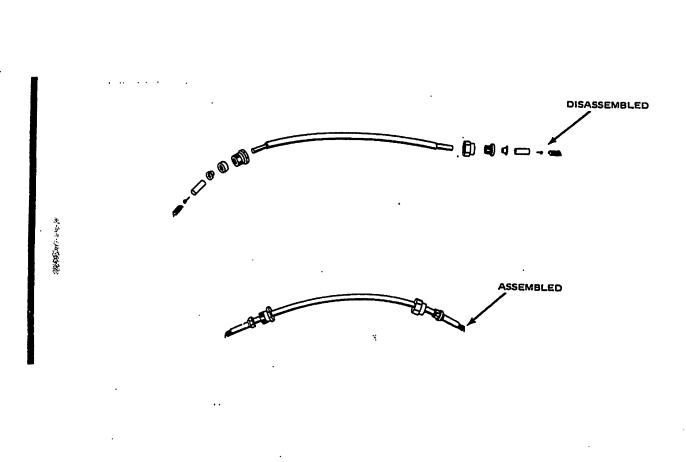
Magneto Lead Arrangement Figure 201
