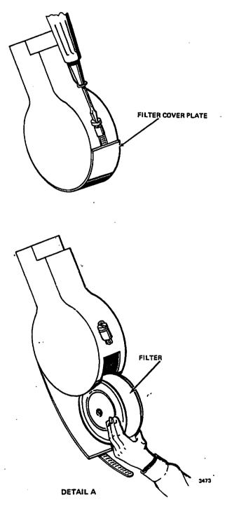
Engine Air Filter Servicing (AA-5B Aircraft) Figure 7
