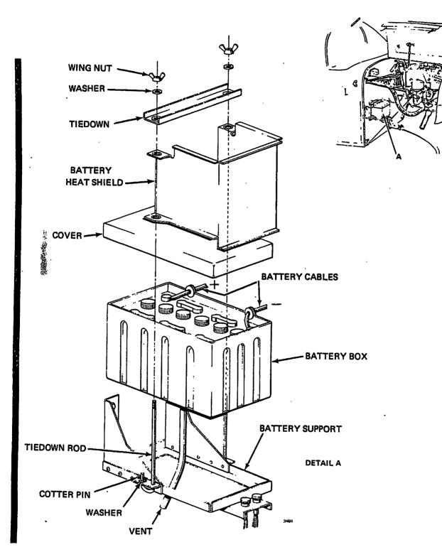
Exploded View of Battery & Battery Box Figure 1
