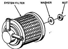
Vacuum System Air Filter Servicing Figure 8
