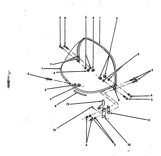
Windshield Assembly Bolt Washer Nut Screw Screw Rivet
