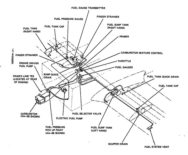
Fuel System Diagram - Models AA-5A (Option) & AA-5B Figure 1 (Sheet 2 of 2) C. The electrical wiring and circuit protective devices that supply electrical power to the auxiliary fuel pump and the fuel quantity indicators is shown in Figure 2.
