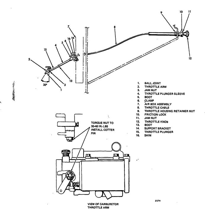
Engine Throttle Control Installation - Model AA-5B Figure 202 .
