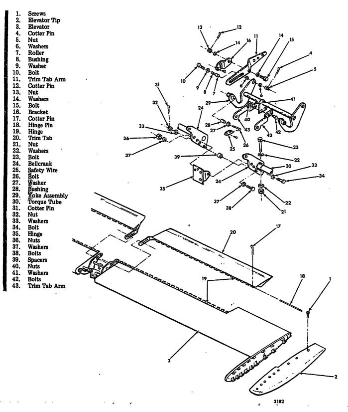
Elevator Disassembly/Assembly (AA-5A and AA-5B Aircraft) Figure 404
