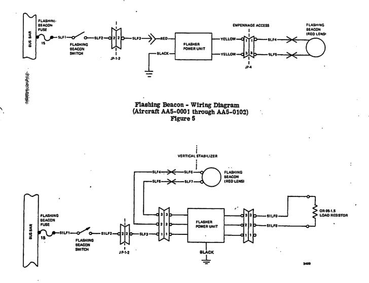
Flashing Beacon - Wiring Diagram (Aircraft AA5-0103 and Subsequent, AA5A-0001 and Subsequent and AA5B-0001 and Subsequent) Figure 6
