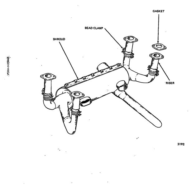
D. Install Exhaust System - AA-5B Aircraft (See Figure 202)
