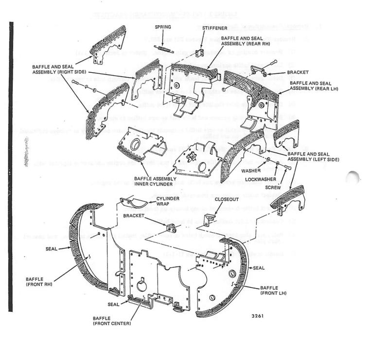
Engine Baffles - AA-5 and AA-5A Figure 201
