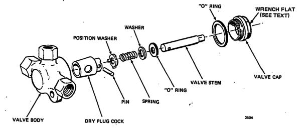
Fuel Selector Valve Disassembly Figure 202
