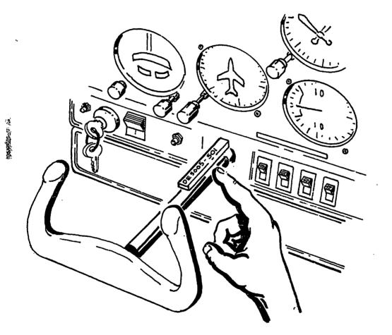
Elevator Rigging Fixture Figure 501
