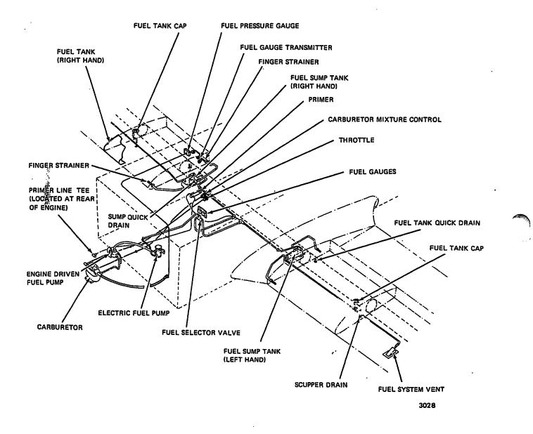
Fuel System Diagram - Models AA-5 & AA-5A (Standard) Figure 1 (Sheet 1 of 2)
