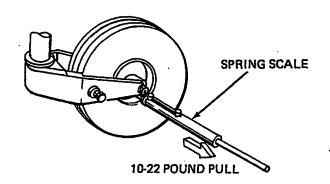
Nose Fork Friction Measurement Figure 202
