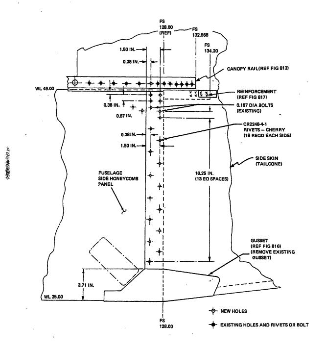
Fuselage Side Attachment Details Figure 814 3417
