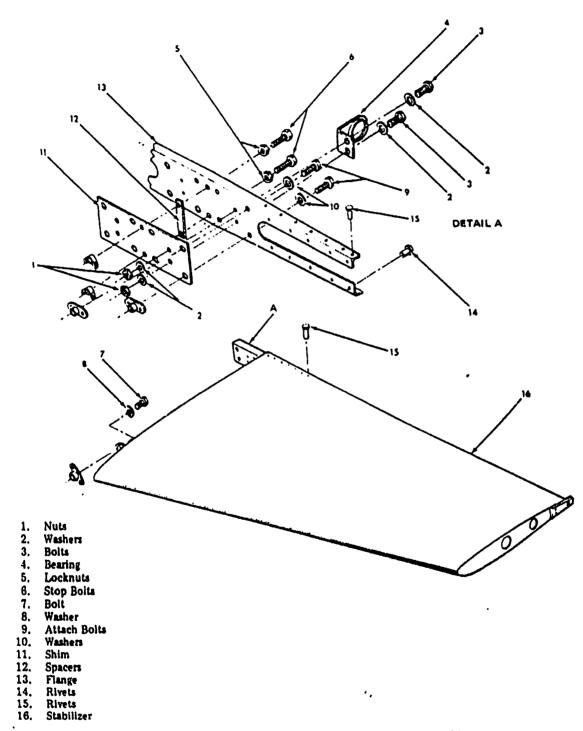
Horizontal Stabilizer Removal/Installation (AA-5 Aircraft) Figure 6
