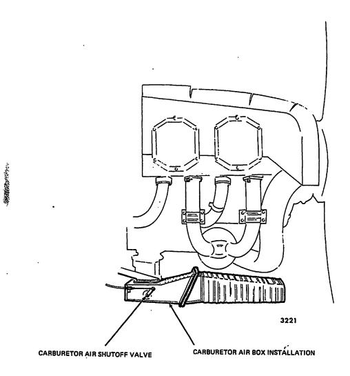
Carburetor Air Box Installation - AA-5 Serial No. 0001 thru 0640 Figure 2
