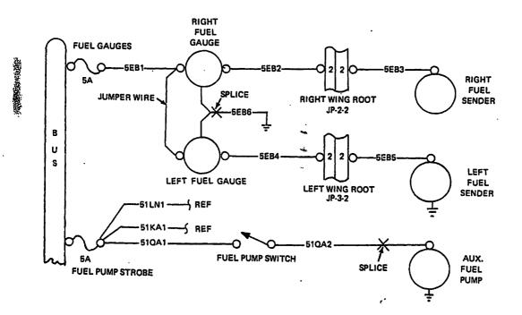
Fuel System Electrical Circuits Figure 2
