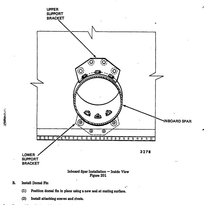
3. Removal/Installation of Dorsal Fin - AA-5 Serial No. 0406 and Subsequent, AA-5A, and AA-5B (See Figure 202.)
