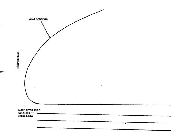
Pitot Tube Alignment Template Figure 202
