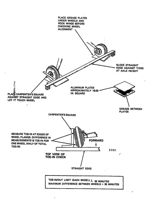
Wheel Alignment Procedure Figure 205
