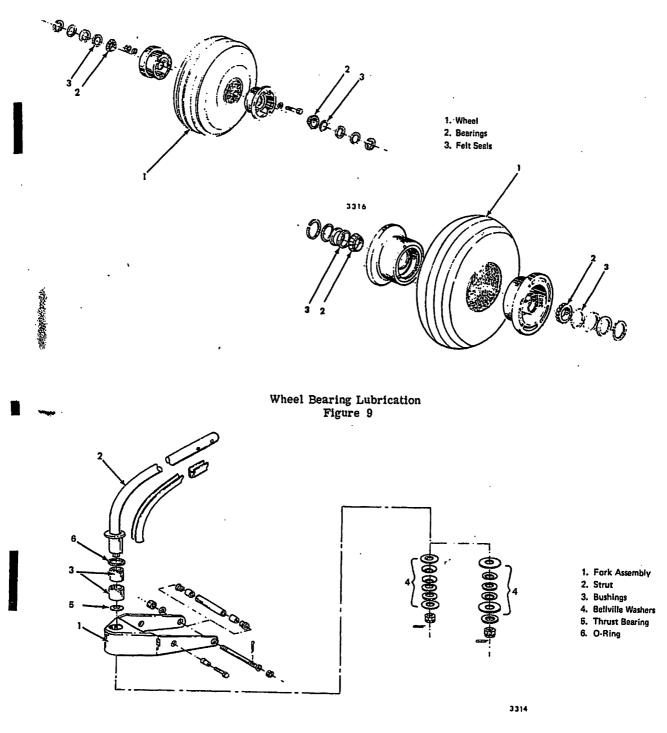
Nose Gear Fork Assembly Servicing Figure 10
