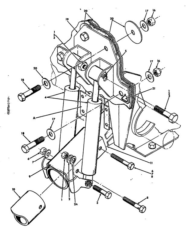
Nose Landing Gear Shock Absorber Installation (Sheet 1 of 2) Figure 203
