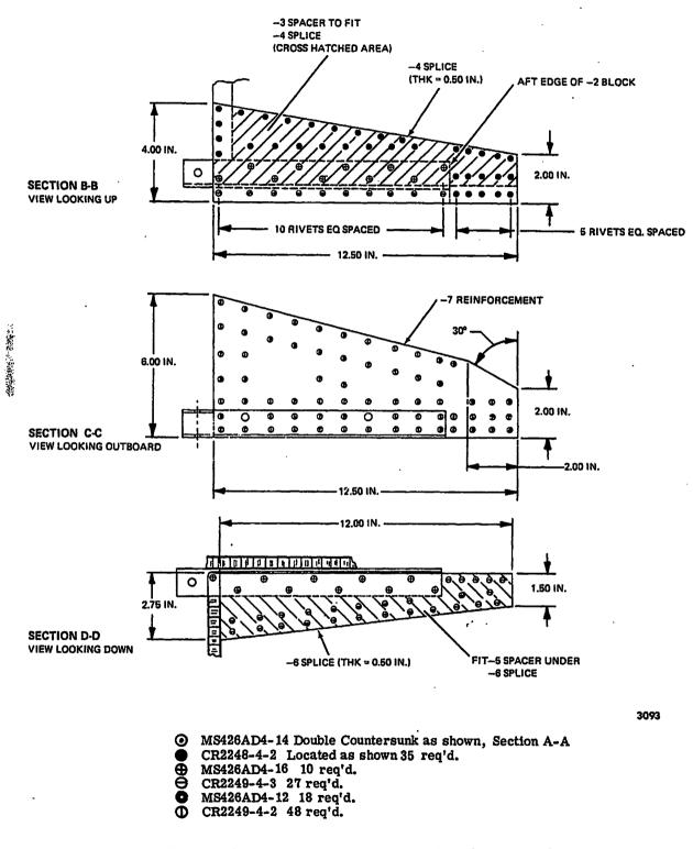
Honeycomb Repair, Lower Engine Mount Area (Sheet 2 of 2) Figure 808
