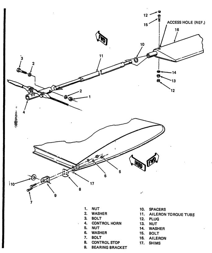
Aileron and Torque Tube Removal/Installation Figure 401
