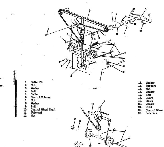
Control Column Removal/Installation Figure 406
