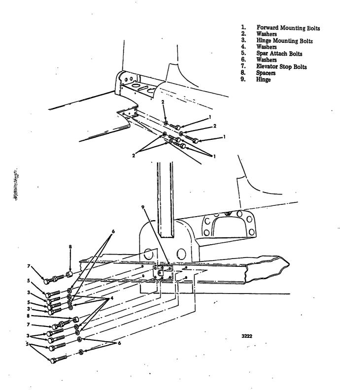
Horizontal Stabilizer Removal/Installation (AA-5A and AA-5B Aircraft) Figure 202
