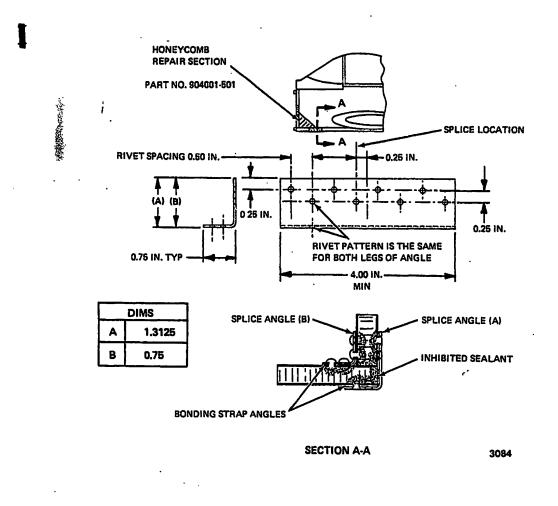
Bonding Strap Angle Splice — (Riveted) Figure 807
