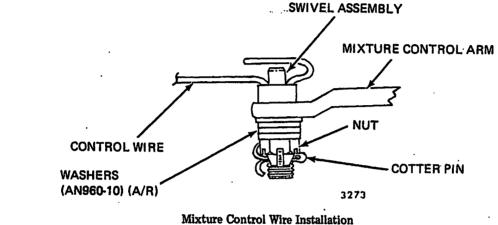
Mixture Control Wire Installation Figure 202
