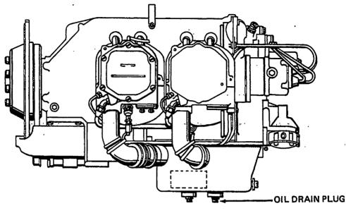
Engine Oil Drain Plug Figure 5
