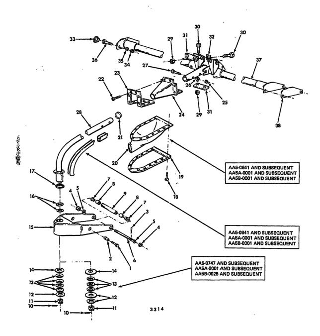
Nose Landing Gear Assembly (Sheet 1 of 2) Figure 201
