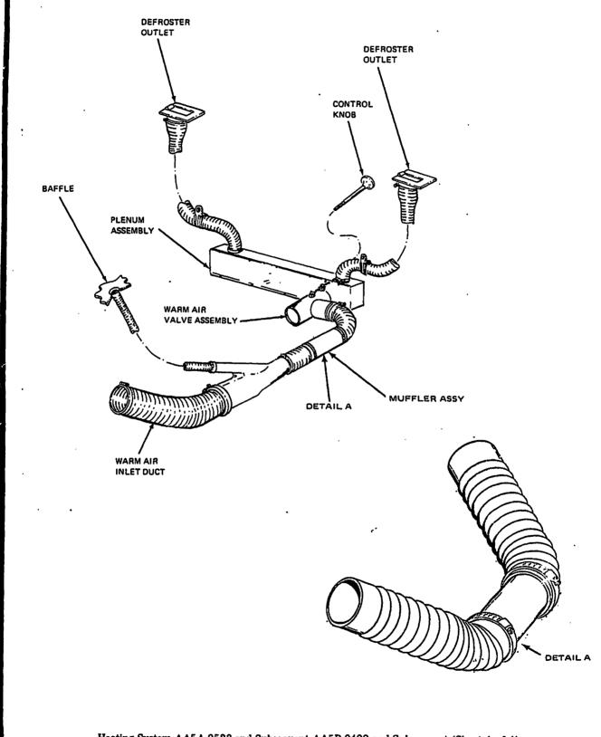
Heating System AA5A-0523 and Subsequent AA5B-0400 and Subsequent (Sheet 4 of 4) Figure 1
