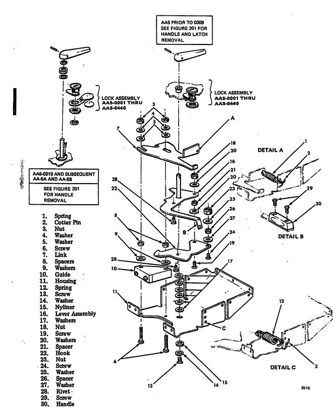
Canopy Latch Disassembly/Assembly (Sheet 1 of 2) Figure 202
