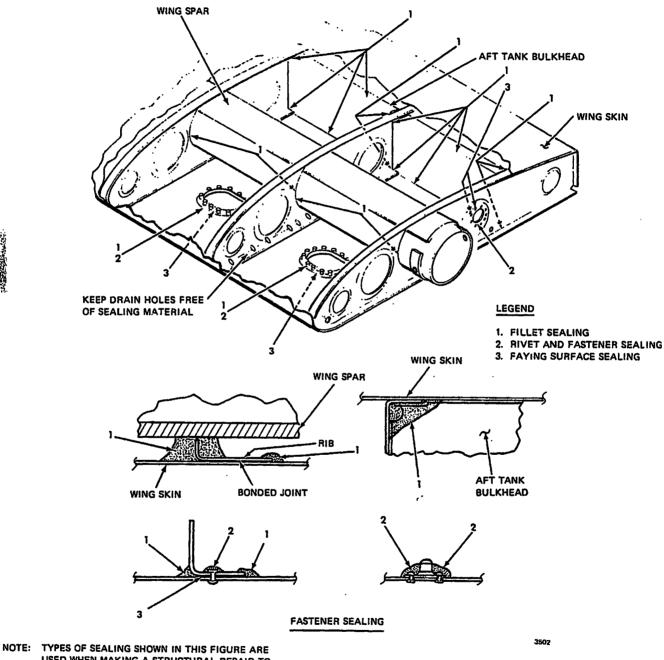
USED WHEN MAKING A STRUCTURAL REPAIR TO THE FUEL TANK AREA AND WHEN REINSTALL-ING THE ACCESS COVERS.
