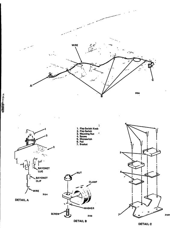
Flap Wiring Removal/Installation Figure 402
