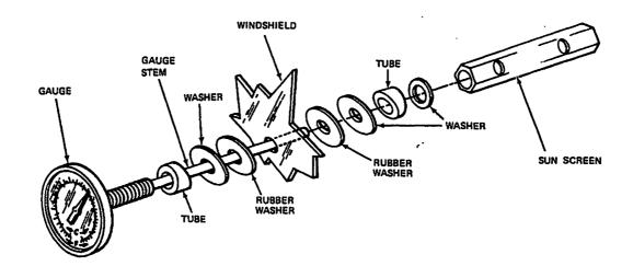
Air Temperature Gauge Installation Figure 201
