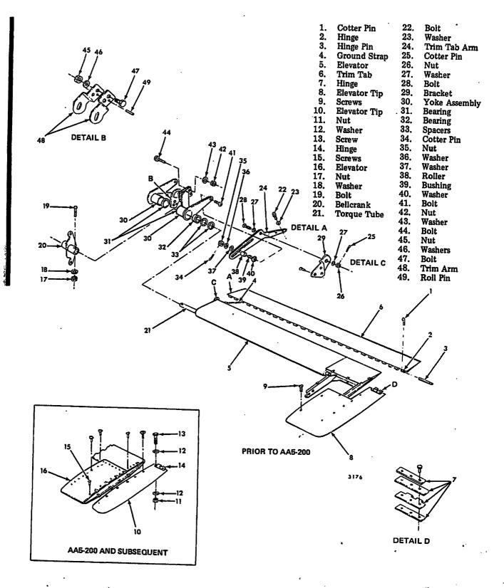
Elevator Disassembly/Assembly (AA-5 Aircraft) Figure 403
