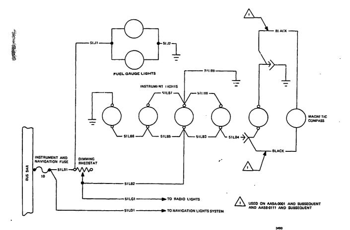
Instrument Lights - Wiring Diagram Figure 1
