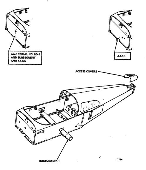
Fuselage Assembly - AA-5 Serial No. 0406 and Subsequent, AA-5A and AA-5B Figure 1 (Sheet 2 of 2)
