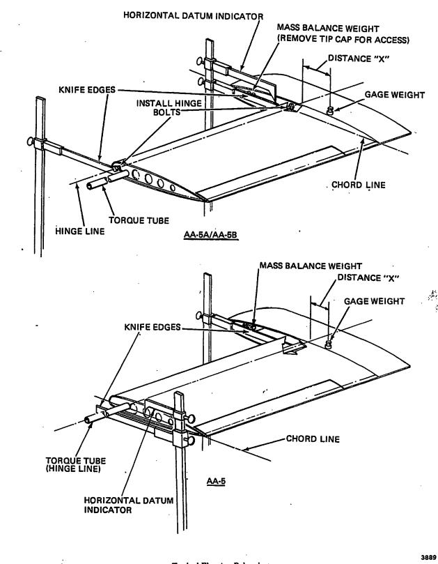
Typical Elevator Balancing Figure 505
