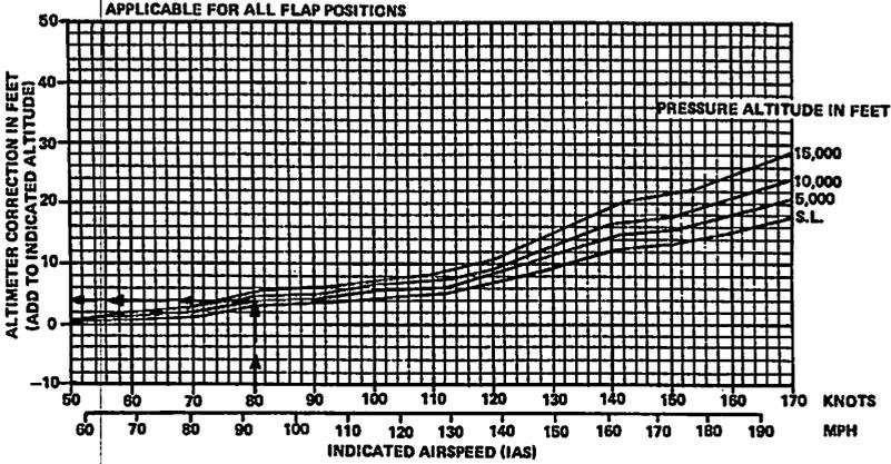
Figure 5-5 Altimeter Calibration
