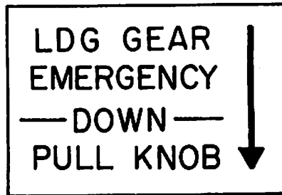
Located on left side of control quadrant
