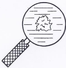
Illustration A Dent or Gouge in a Blade Face
